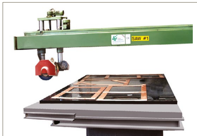
Example of model positioning before cutting the slab
